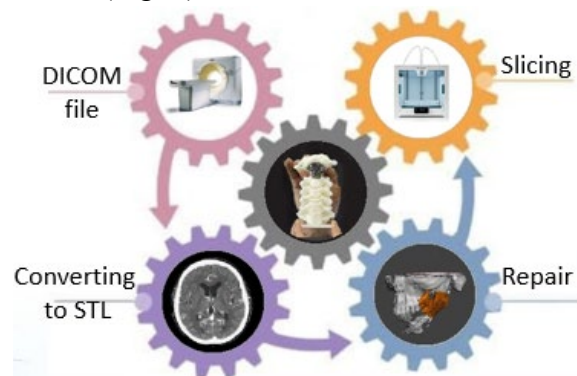
Figure 1. Process of 3D printing of medical models
